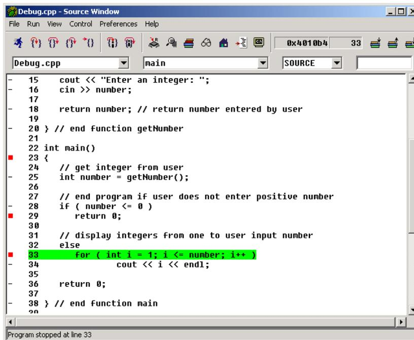
Fig. 1.28 `Debug.cpp` halted at line 33.
